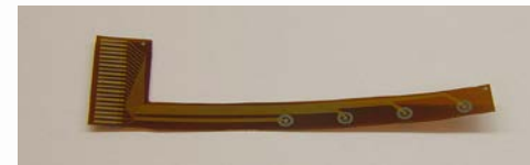
Flexible sensor strip for wearable biomedical monitoring
